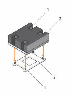
Figure 39. Removing and installing a processor heat sink
